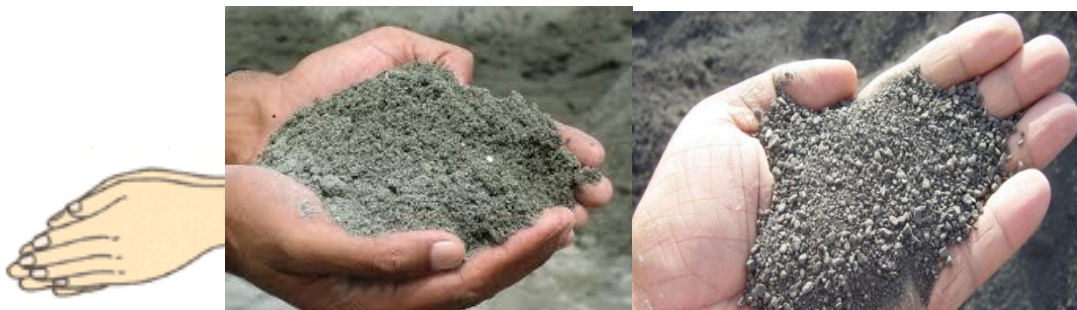
Testing of CS-Sand by "visual observation" and "rubbing with hand" to assess the presence of Quarry dust
