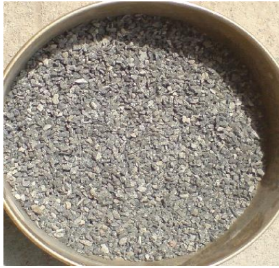
Poor Quality CS-Sand with Flaky Particles
