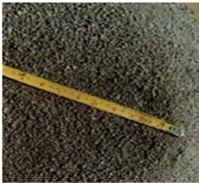
VSI Crushed Sand - Cubical - Good Quality
